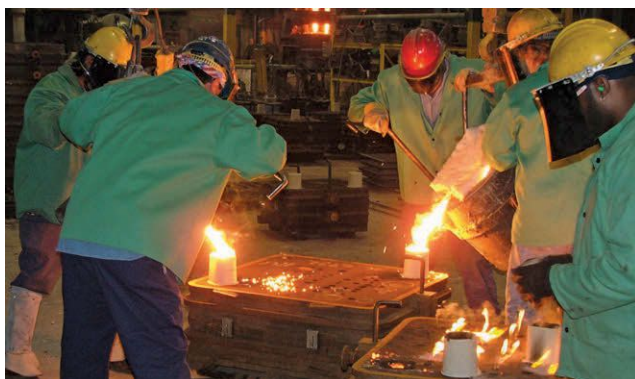
These molten metal handlers are protected with full face shields, gloves, and coats.
