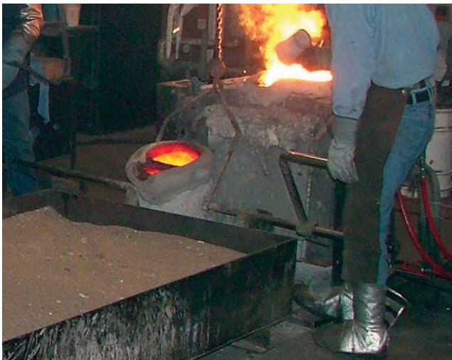
Protective footwear is important to keep molten metal and sparks from lodging in boots.
