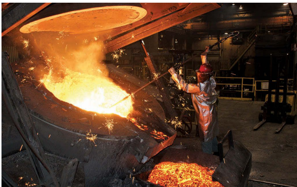
Certain PPE is required to protect the body from head to toe in melting operations.
