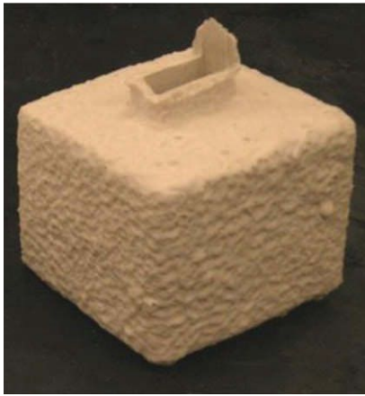
Fig. 1. This investment casting shell was built around a foam pattern.
