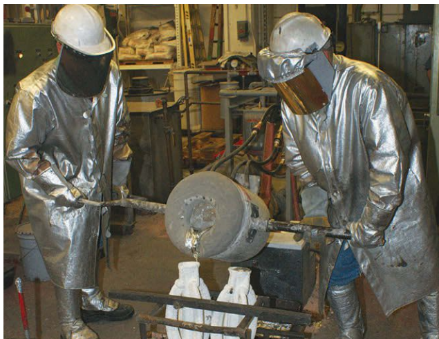
Proper melting gear can include boots, coats, face masks and hard hats.
