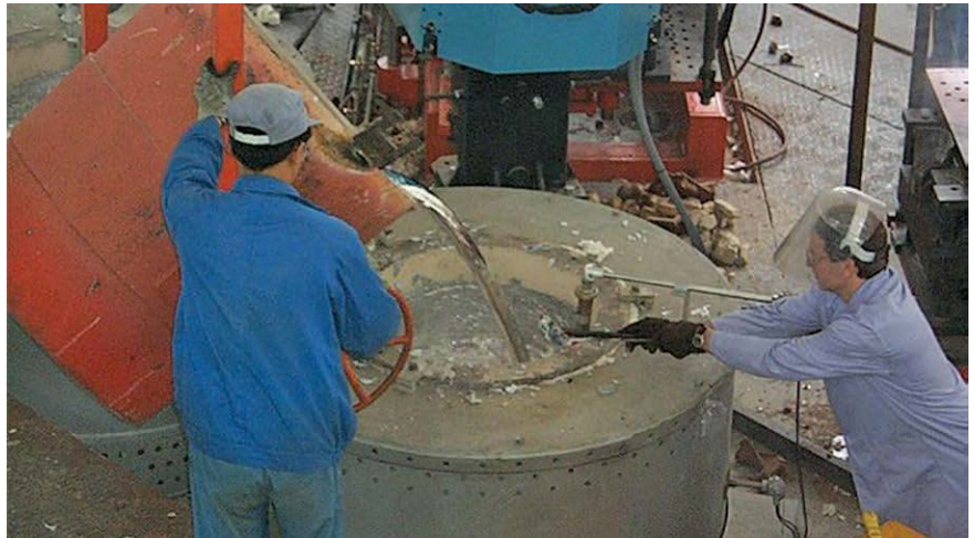
A bull ladle and crane system can be utilized to move large volumes of metal from the primary melting furnace to the casting furnace.
