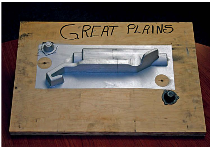
Kansas Castings produced 40 castings using the plastic pattern Great Plains produced on its 3D printing machine.
