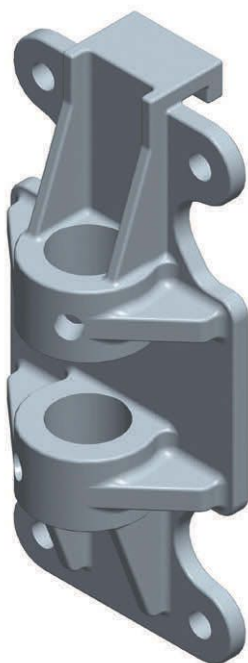
The initial quick-attach mount model was designed with four bolt holes.
